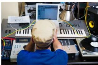
These are musical instruments connected to a computer using a musical instrument digital interface (MIDI). The interface converts the output signals from the instrument into a digital form understood by the computer.
