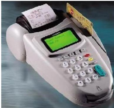
These are a type of smart card reader, but tend to be used only at EFTPOS terminals. There are a number of versions of these readers.
