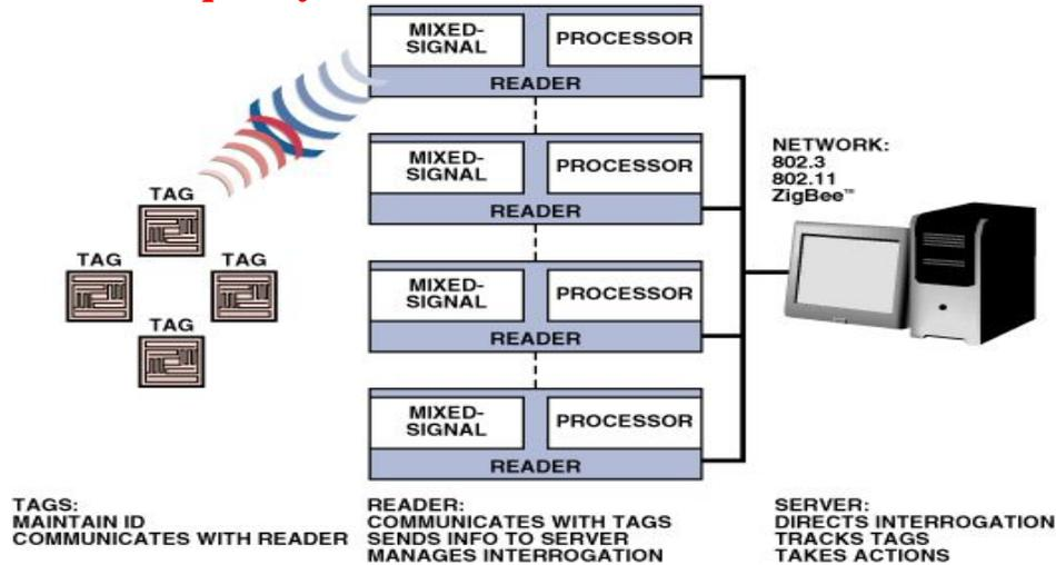
Radio frequency identification (RFID) tags are attached to objects so that the object can be identified through the use of radio waves.
