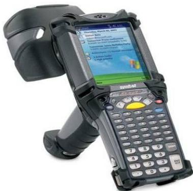
The reader is used to transmit a radio signal in order to communicate with the RFID tag. It then uses the data it receives to identify the object. Some are handheld and some — called portals — are used at doors to detect objects passing through the doorway or entrance or exit to a building.
