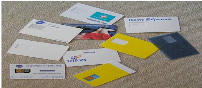
Smart cards are often referred to as chip cards. They are similar in appearance to a magnetic strip card, but information is stored on a chip on the card. This can be used for storing a PIN and/or other personal data.
