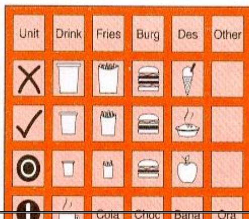
Concept keyboards are used when fast input is needed and are ideally suited to selecting from a limited range of choices
