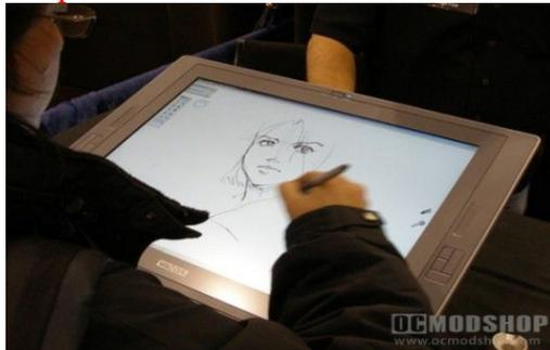
Graphics tablets are used together with a stylus to trace round maps or hand-drawn images. As they are traced round, the resulting images appear on the computer screen. They can then be stored for further use.
