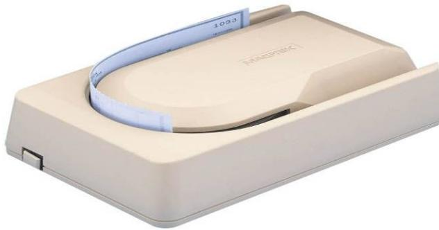
Magnetic ink character recognition (MICR) is the system used in the processing of bank cheques.
