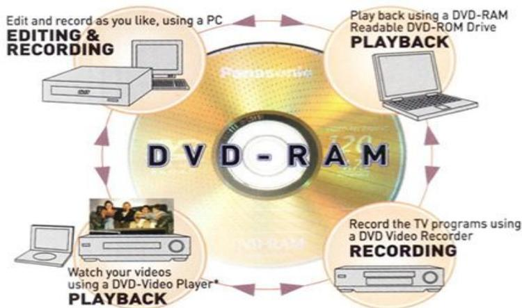
The digital versatile disk random access memory (DVD RAM) is a newer technology. The recording surface is an alloy coating, as with DVD RWs. However, **the data is stored in concentric tracks like magnetic media, unlike the single spiral of a single track that is used in other optical media.**
